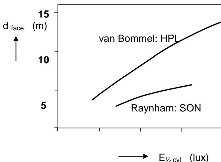
**Figure 3** Identification distance  $d$ , under residential area lighting circumstances in dependence of semi-cylindrical illuminance  $E_{1/2cyl}$ , with white high pressure mercury light HPL and with yellowish high pressure sodium light. Raynham [8].
