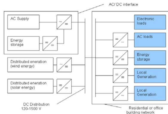
**Figure 1** LVDC network with distributed generation units [1]
