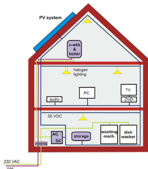
Figure 3 AC and DC low voltage hibrid system [3]
