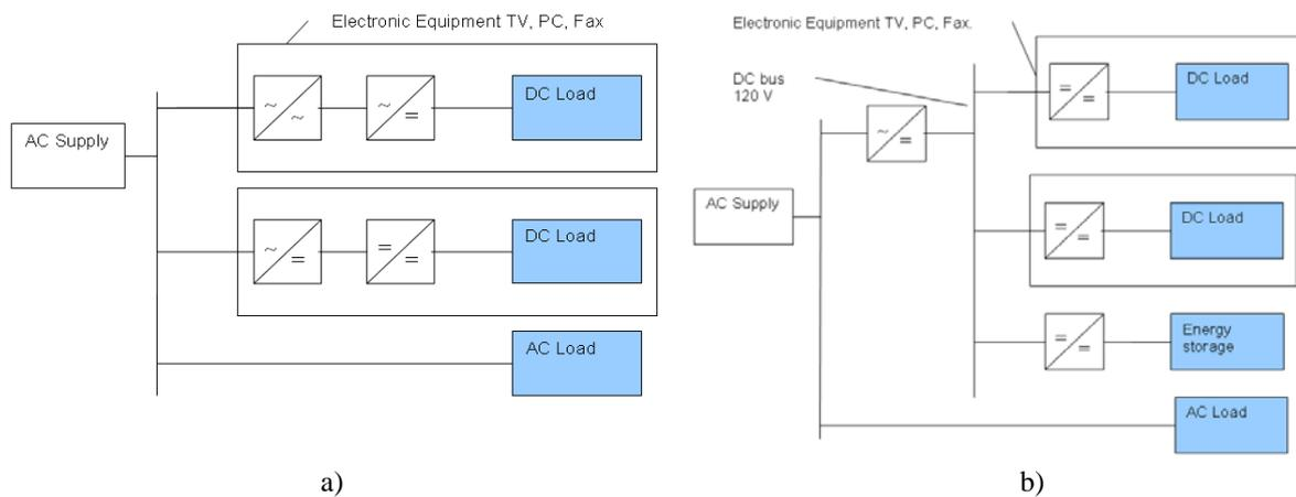
**Figure 2** a) AC voltage Supply and b) AC and DC Voltage Supply [2]
